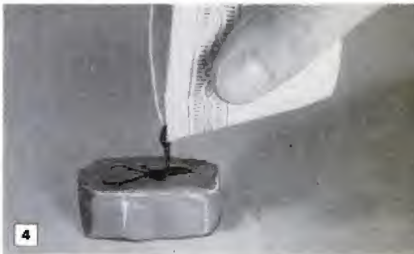
Liquid-plastic solution is mixed with catalyst and dye and then poured slowly into rubber mold, above. After hardening and cooling, inlays are cemented to handle tang, below
